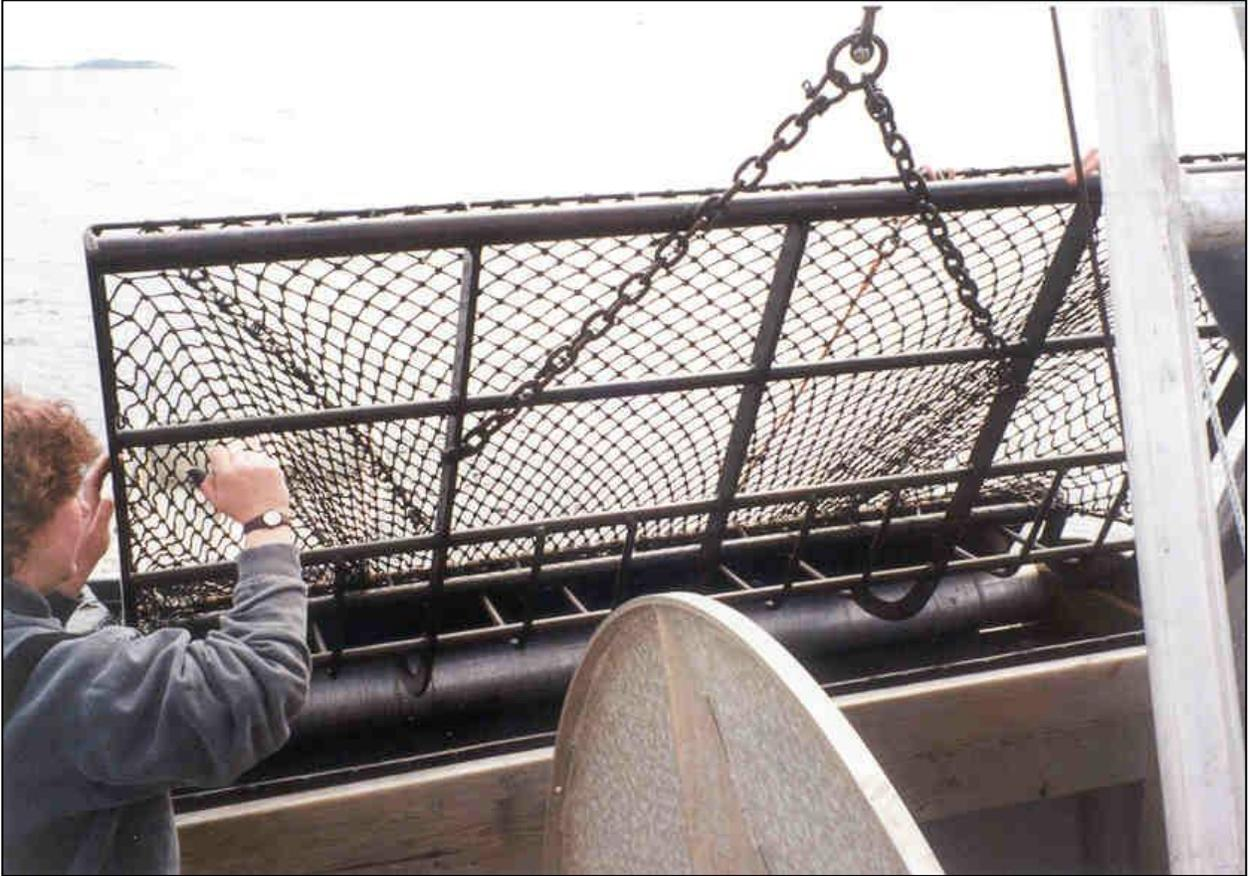
Figure 3. Photo of the off-bottom butterfly trawl used in the Pacific scallop trawl fishery (Photo credit, DFO)
